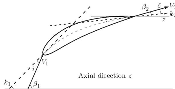
Fig. 3. The correlations between cascade and aerodynamics parameters
